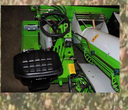
All important maintenance items are easily reachable. The hydraulic drive sytem ensures low operation and maintenance costs for a long time
