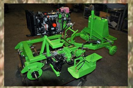
The fexibly displacable side raker (optional equipment) works gently and is also very adaptive. Drive system, excavation and crossdisplacement are driven hydraulically
